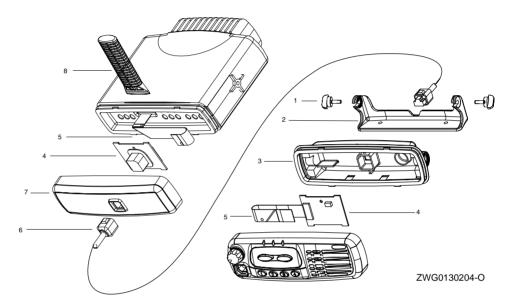
Figure 1-8 Remote Front and Back Housings
