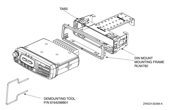
Figure 1-6 Mounting the Radio into the Dashboard
