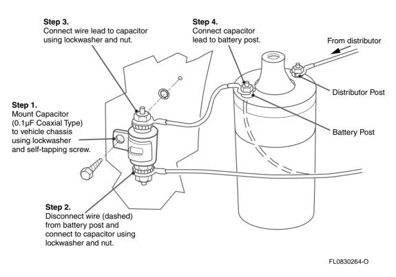
Figure 2-5 Ignition Coil Noise Suppression
