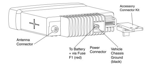
Figure 1-4 Connections to the Back of Radio
