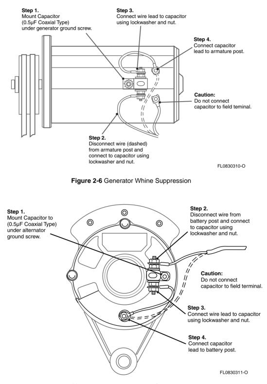
Figure 2-7 Alternator Whine Suppression
