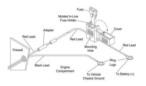
Figure 1-2 Power Cable Assembly
